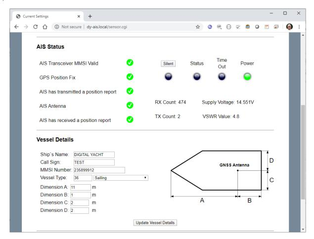
A series of simple Tick and Cross icons give an immediate indication of correct operation and you also have the RX and TX count to show how many targets have been received and how many successful transmissions the iAIS TX has made.
