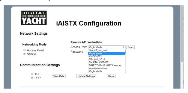
By default, the iAIS transmits wireless NMEA data in UDP mode which is the easiest mode to setup in most apps – just tell the app that the UDP data is on port 2000 and it should start receiving data. In some apps, such as the popular Navionics Boating app, the iAIS TX will even be detected automatically and no app setup is required.
