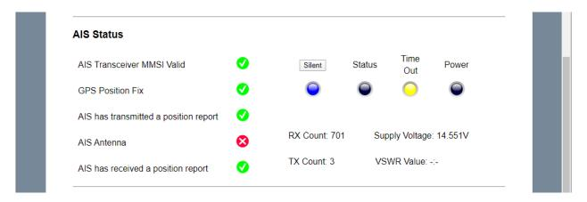
To start transmitting again, simply click the "Silent" button again and the blue "Silent" LED will go off and as soon as the iAIS TX makes its next transmission the green "Power" LED should illuminate, and this indicates that everything is working correctly, with all self-tests passed.
